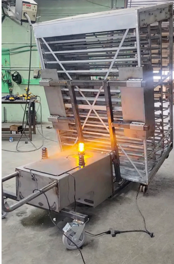
Jamesway 3 column rack being tilted
